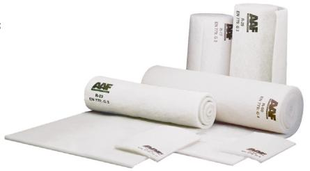
R-series air filter media is made of synthetic fibres, except type R20 Natural, which is made of natural fibres. An exclusive bonding technology ensures a high number of fibres per square metre for a given weight.
